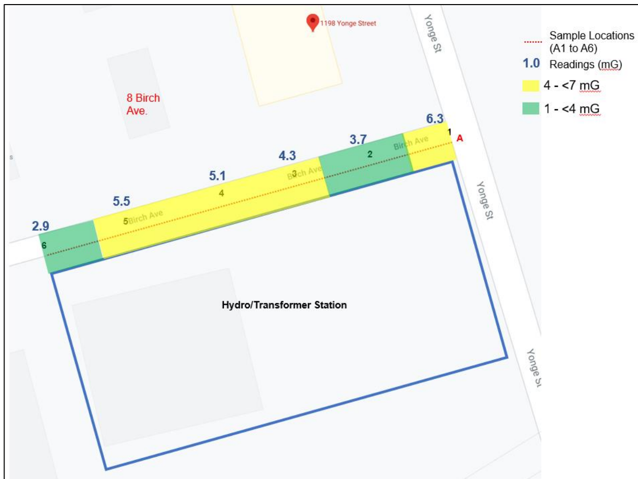
Figure 2-3 Magnetic Field Level Contours for the Adjacent Hydro/Transformer Station
