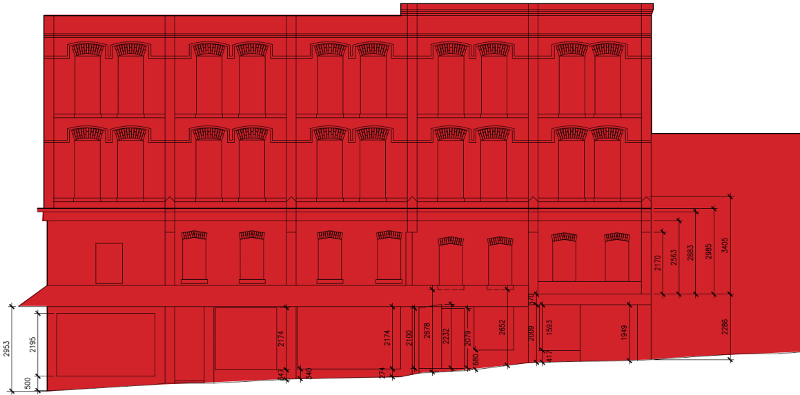
Existing east (principal) elevation of Building A with proposed demolition indicated in red (ERA, 2021).
